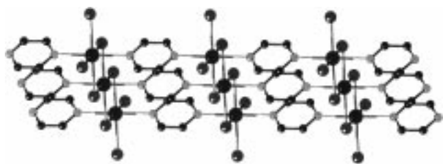
Figure 36. The layer structure of [\text{Cd}(\text{pz})\text{Cl}_2] .
